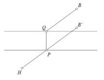
This distance is minimal since HP+PQ+QB = HP+PQ+PB0. PQ = w is constant, and HP+PB0 is clearly minimized when P is on the straight line HB0.
