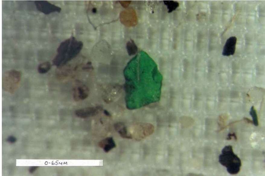
Figure 8. Example of an 'exotic' synthetic Cr-rich particle identified by optical microscopy, interpreted to be of 'industrial' origin.
