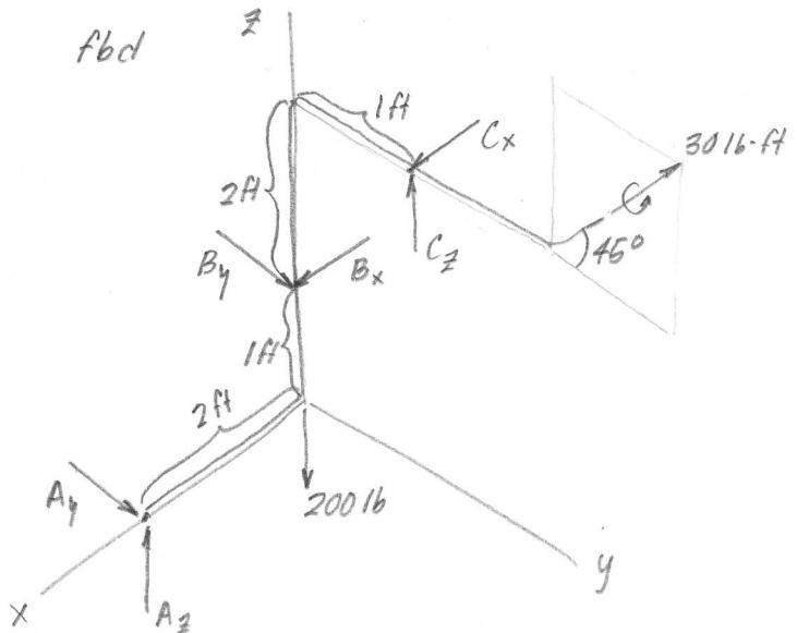
$$\begin{aligned}\sum \vec{M}_A = 0, \quad & -2i(f) \times -200k(lb) \\ & + (-2i + 1k)(A) \times (B_x i + B_y j) \\ & + (-2i + 1j + 3k)(A) \times (C_x i + C_z k) \\ & + 30 \cos 45^\circ j(lb \cdot ft) + 30 \sin 45^\circ k(lb \cdot ft) = 0\end{aligned}$$
