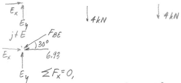
$$10.393 \text{ kN} - 6.93 \text{ kN} - F_{BE} \cos 30^\circ = 0 \\ F_{BE} = 4 \text{ kN (C)} \quad (1.5)$$
