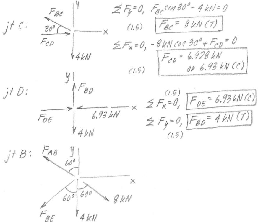
$$\sum F_y = 0, F_{BC} \sin 30^\circ - 4 \text{ kN} = 0 \quad (1.5) \\ F_{BC} = 8 \text{ kN (T)}$$
