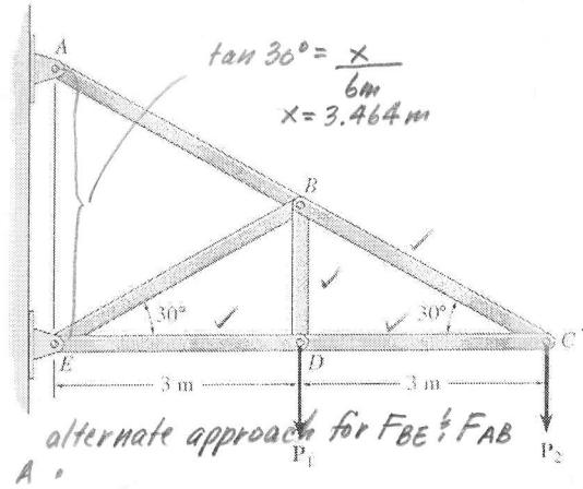
$$\sum M_A = 0, E_x(3.464 \text{ m}) - 4 \text{ kN}(3 \text{ m}) - 4 \text{ kN}(6 \text{ m}) = 0 \\ E_x = 10.393 \text{ kN} \quad (1)$$
