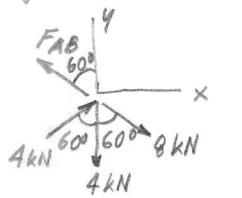
$$\sum F_x = 0, -F_{AB} \sin 60^\circ + 4 \text{ kN} \sin 60^\circ + 8 \text{ kN} \sin 60^\circ = 0 \\ F_{AB} = 12 \text{ kN (T)} \quad (1.5)$$
