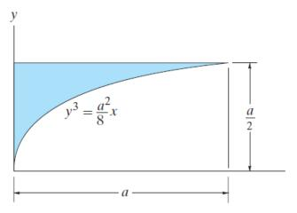
2. Determine the moment of inertia of the composite area about the y-axis (the area is symmetric about the y-axis).
