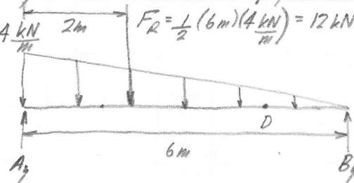
$$\sum M_A = 0, -(12 \text{ kN})(2\text{m}) + B_y(6\text{m}) = 0 \\ B_y = 4 \text{ kN}$$
