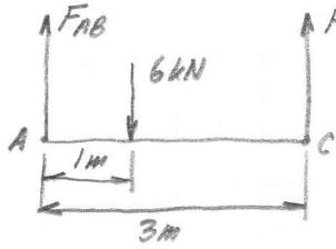
$$\sum M_A = 0, -(6 \text{ kN})(1 \text{ m}) + F_{CD}(3 \text{ m}) = 0, F_{CD} = 2 \text{ kN}$$
