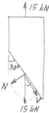
$$N = 15 \text{ kN} \sin 30^\circ = 7.5 \text{ kN}$$
