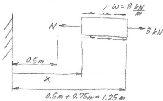
$$\sum F_x = 0, -N + 8 \frac{\text{kN}}{\text{m}} (1.25\text{m} - x) + 3 \text{ kN} = 0$$
