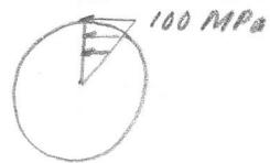
$$T_{max} = \left(100 \times 10^3 \frac{kN}{m^2}\right) \frac{\frac{\pi}{2} ((0.050m)^4 - (0.0375m)^4)}{(0.050m)} = 13.42 \text{ kN-m or } 13.4 \text{ kN-m}$$
