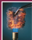
Steel wool heated in air (about 20% O 2 ) glows red-hot but oxidizes to Fe 2 O 3 slowly.
