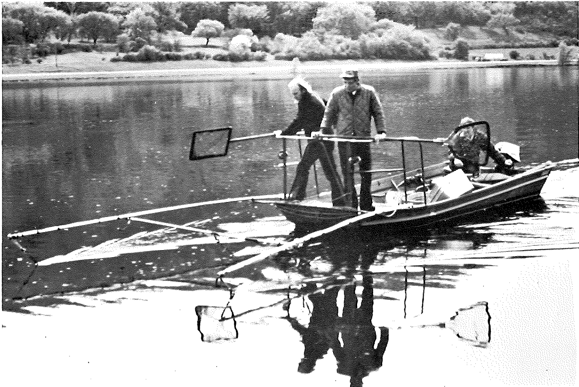
Figure 11-1. Minnesota Department of Natural Resources lake survey crew using electrofishing equipment to sample fish populations.
