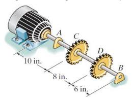
2. The tubular shaft of the motor shown below has an outer diameter of 20 mm and a wall thickness of 2.5 mm and is made of a material with an allowable shear stress of  $\tau_{\text{allow}} = 75 \text{ MPa}$ . Determine the maximum allowable power (in kW) that can be supplied when the shaft is operating at 1,500 rpm.
