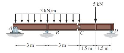
(2) Draw the shear and moment diagrams for the beam. Make sure you provide the applicable values on the diagrams (at the beginning/end and where any transitions occur).
