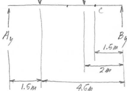
$$\sum M_A = 0, -(1.5\text{m})(30\text{ kN}) - (4\text{m})(15\text{ kN}) + (6\text{m})B_y = 0$$
