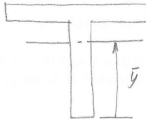
$$\bar{y} = \frac{(0.165\text{ m})(0.150\text{ m})(0.030\text{ m}) + (0.075\text{ m})(0.030\text{ m})(0.150\text{ m})}{(0.150\text{ m})(0.030\text{ m}) + (0.030\text{ m})(0.150\text{ m})}$$
