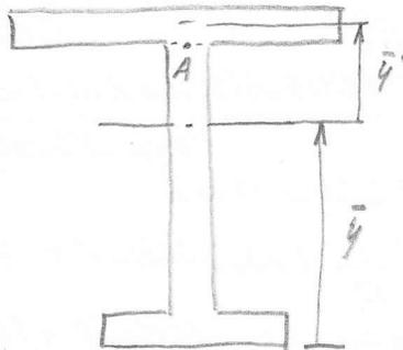
$$\bar{y} = \frac{(0.295\text{m})(0.200\text{m})(0.030\text{m}) + (0.155\text{m})(0.025\text{m})(0.250\text{m}) + (0.015\text{m})(0.125\text{m})(0.030\text{m})}{(0.200\text{m})(0.030\text{m}) + (0.025\text{m})(0.250\text{m}) + (0.125\text{m})(0.030\text{m})}$$
