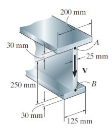
(2) Determine the maximum shear stress in the beam at point C.
