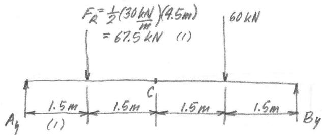
$$\sum M_A = 0, -(67.5 \text{ kN})(1.5 \text{ m}) - (60 \text{ kN})(4.5 \text{ m}) + B_y(6 \text{ m}) = 0$$
