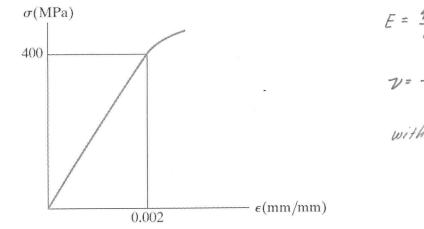
$$E = \frac{400 \text{ MPa}}{0.002 \text{ MMM}} = 200 \text{ GPa} \quad (2)$$
