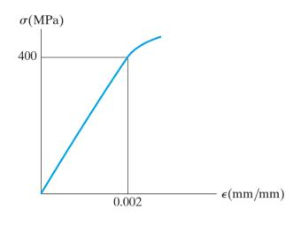
2. Below is a steel column (in black) with an 18 in<sup>2</sup> cross-sectional area. The steel column is encased in concrete (in gray) to the dimensions shown. An axial force of 60 kip is applied to the column. What is the average compressive stress in the steel and the average compressive stress in the concrete? By how much does the 8 ft column shorten? The modulus of elasticity of the steel is  $29 \times 10^3$  ksi and the concrete is  $4.20 \times 10^3$  ksi.
