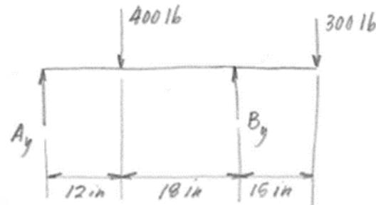
$$M_A = 0, -(12\text{ in})(400\text{ lb}) + (30\text{ in})B_y - (45\text{ in})(300\text{ lb}) = 0$$
