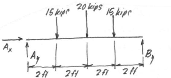
$$\sum M_B = 0, \quad (2\text{ft})(15\text{kips}) + (4\text{ft})(20\text{kips}) + (6\text{ft})(15\text{kips}) - (8\text{ft})A_y = 0 \\ A_y = 25 \text{ kips}$$
