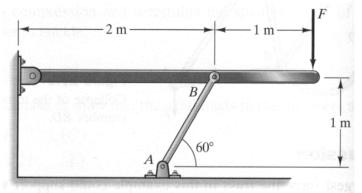
2. Determine the stress components acting on plane AB.
